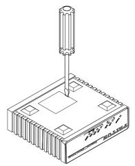
Figure 8. Removing protective cover
